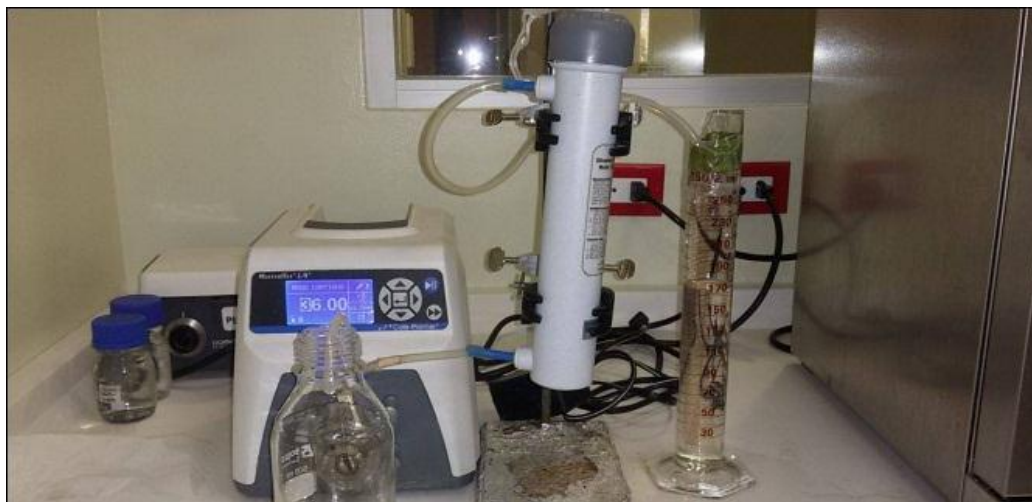
Figura 5. Reactor Continuo (Cole-Parmer Master Flex L/S Digital Drive Model 7523-80) Fuente. Autora
