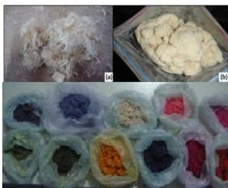
**Figure 4.** Unmilled (a), milled 1 mm long (b) agave and dyed milled fiber (c).
