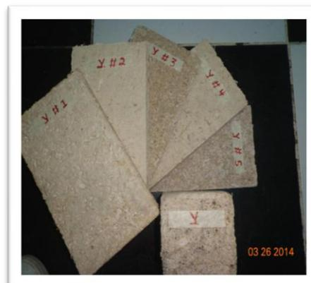
Fig.5.5 Probetas yeso-bagazo
