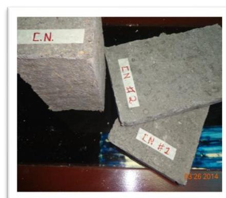
Fig. 5.6 Probetas cemento-ceniza-bagazo
