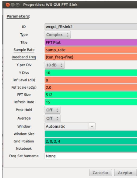
Figura D.19. Bloque **FFT Sink** del receptor FM.
