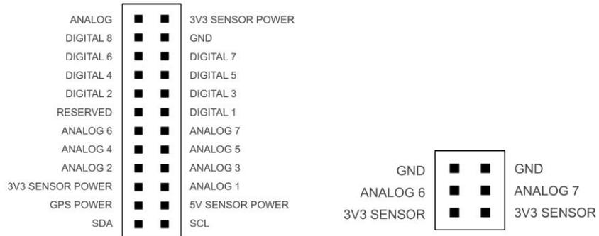
Figure 34: Description of sensor connector pins
