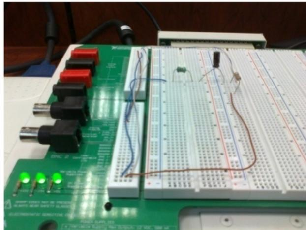
Fig. 5.11 Red inductor-capacitor-resistor
