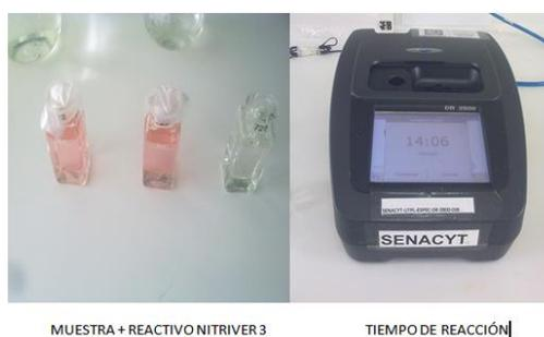
Figure 44 Reaction of nitrite
