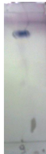
Figure3. Chromatogram revealed the fraction LF9. Stationary phase: Silica gel. Mobile phase: Hex-EtOAc (1:1)
