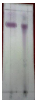
Figure1. Chromatogram revealed the fraction LF7, and its mother liquor. Stationary phase: Silica gel. Mobile phase: Hex-EtOAc (1:1)
